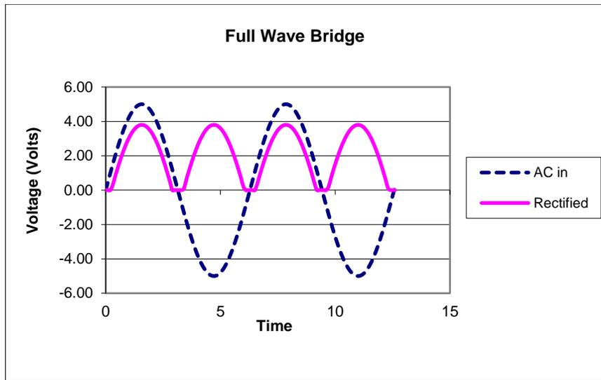
of the full wave bridge. This will produce an output that looks like fig. 7.13 with the original rectified signal shown as well and fig. 7.14 with just the filtered signal. These assume that there
