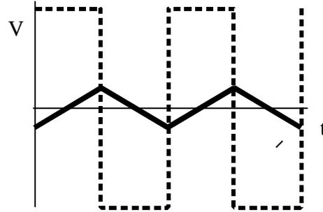
Fig. 7.11 Oscillator Output (dashed line)
