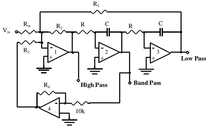
Fig. 6.7 State Variable Filter
