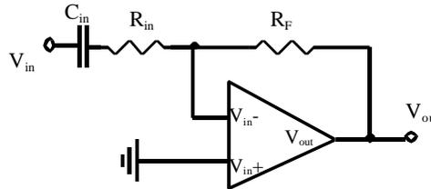
Fig. 6.2: High Pass Filter
