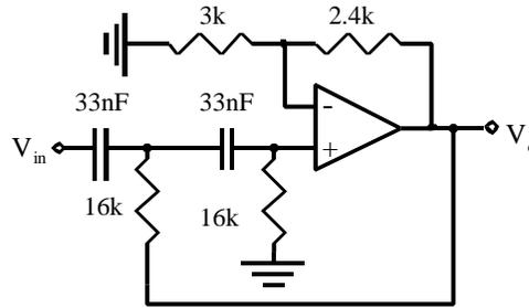
Fig. 6.5: Sallen-Key High Pass Filter
