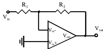
Fig. 5.3: Inverting Amplifier
