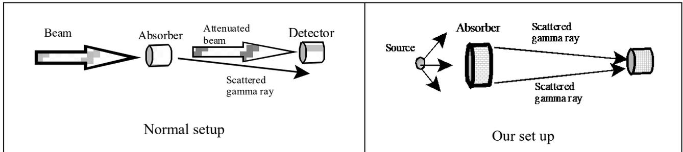
(spherically symmetric). The absorber has a large area, so photons scattered through moderate angles can still strike the detector which is also fairly large. Their energies may overlap the lower edge of the photopeak, blurring out that part of the photopeak. However, we do not want to count those if we want to measure only the ones that get through unscathed. In that case, the net count may yield a better measurement of the attenuation length than the gross count. (Why?)
