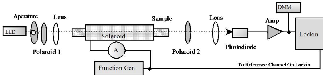
Setup for Measuring the Verdet Constant using an LED
