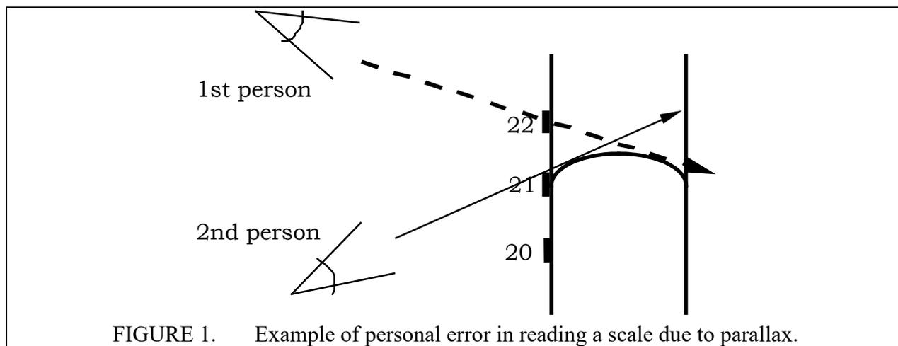
FIGURE 1. Example of personal error in reading a scale due to parallax.
